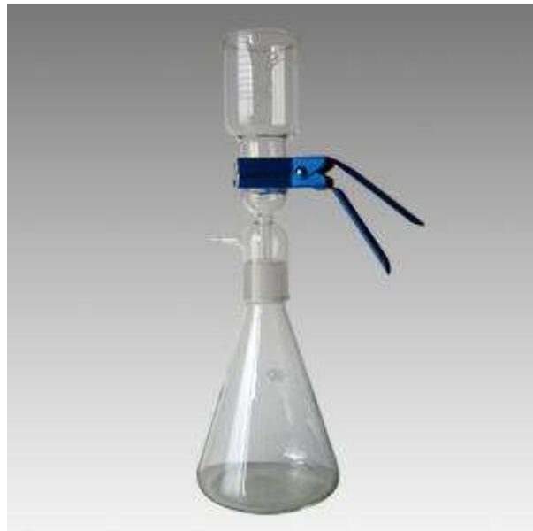
Figure 1-2: Suction filtration system with membrane holder
